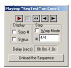
5. Click Unload the Sequence to stop running the sequence, and to return the generator to normal operating mode.
